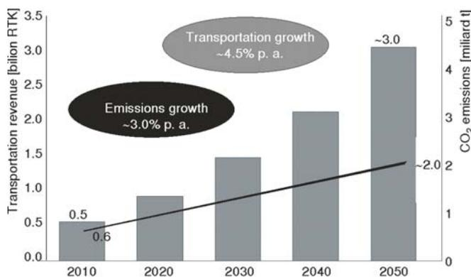
Figure 4. “Base case” prediction for the transportation and CO<sub>2</sub>-emissions growth in the aviation sector [6]
