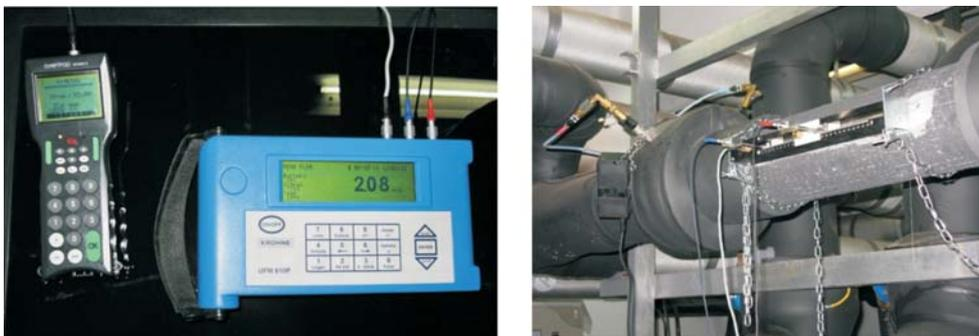
**Figure 9. Instrument OVENTROP OV-DMC 2 and ultrasonic flow-meter KROHNE UFM 610P**
