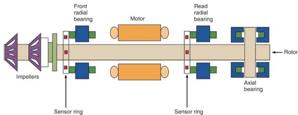
**Figure 5. Schematic diagram of basic compressor elements**
