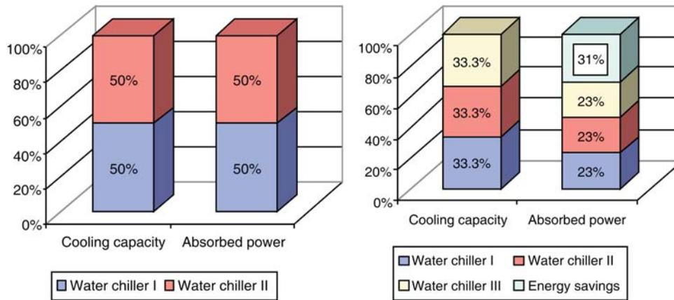
**Figure 6. Comparative presentation of energy consumption, if two or three water chillers are operational for the same total cooling capacity**
