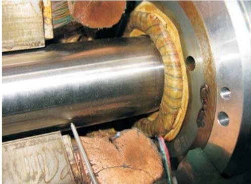
**Figure 4. Electromagnetic compressor bearing**
