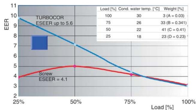
**Figure 2. Energy efficiency ratio of water chiller at different loads**
