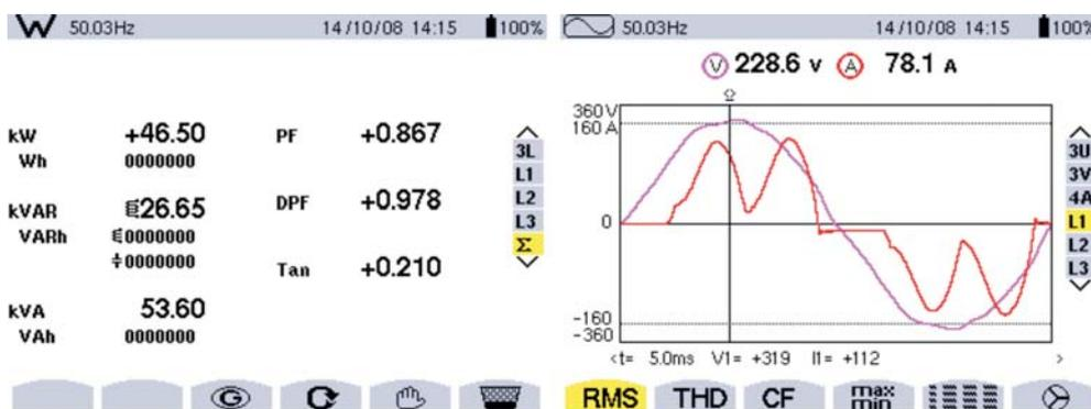
**Figure 10. Results of the electrical parameters measuring (power,  $\cos\varphi$ , voltage, current intensity)**
