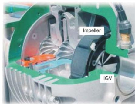
**Figure 3. Cross-section of Turbocor compressor** (full color figure is available in electronic version)
