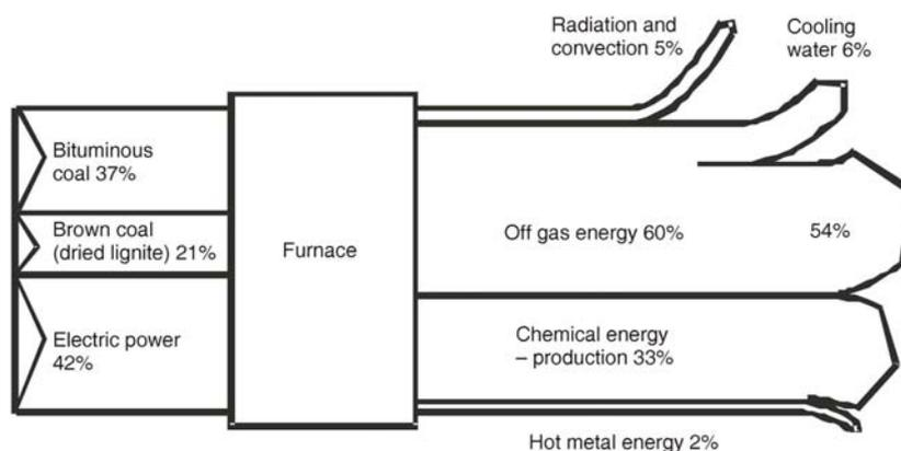
Figure 3. Rough Sankey diagram of the energy flow in the furnace No. 7
