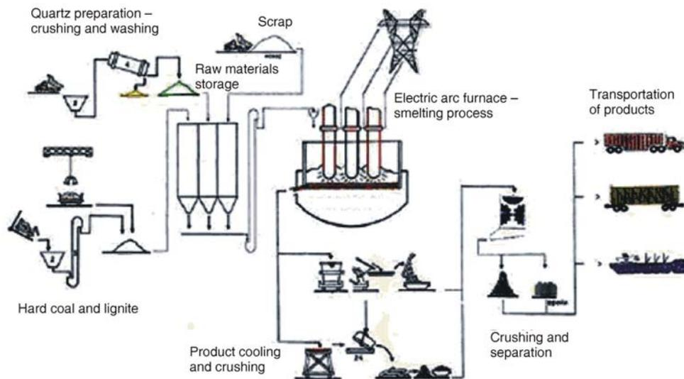
Figure 1. Main operations in the production process [6]
