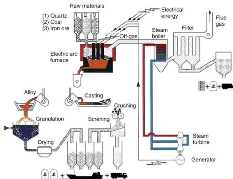
Figure 4. Process flow diagram for a modern production of ferro-silicon and silicon metal [5]
