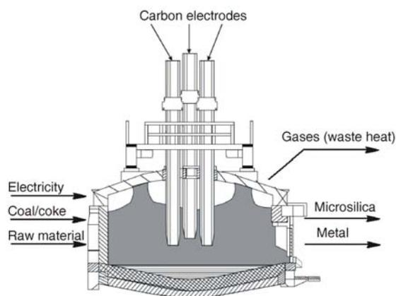
Figure 2. Typical design of submerged electric arc furnace (EAF)
