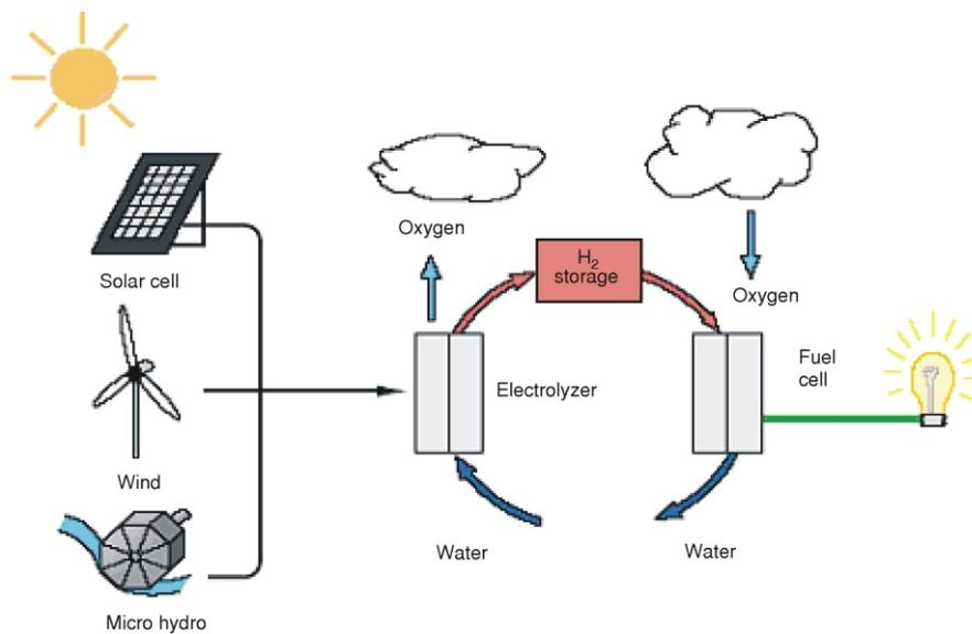
**Figure 4. Renewable energy storage by the use of fuel cell**
