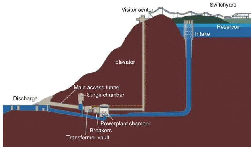
**Figure 1. Schematic of a pumped water storage plant**
