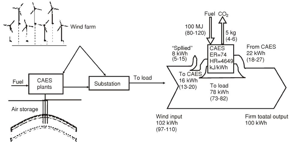
**Figure 2. Wind/CAES energy storage arrangement and its energy balance**
