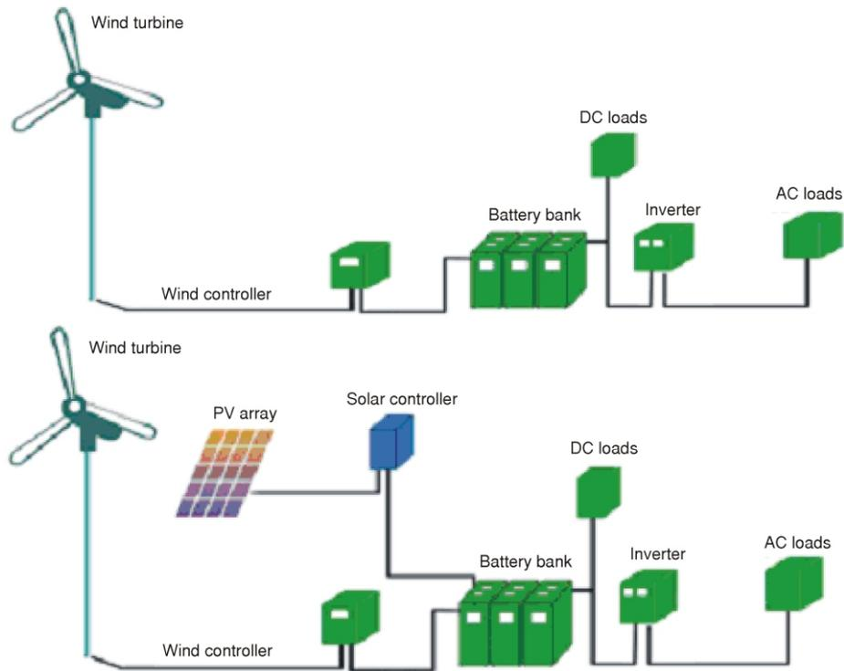
**Figure 3. Small scale wind and wind/solar hybrid systems with battery storage**
