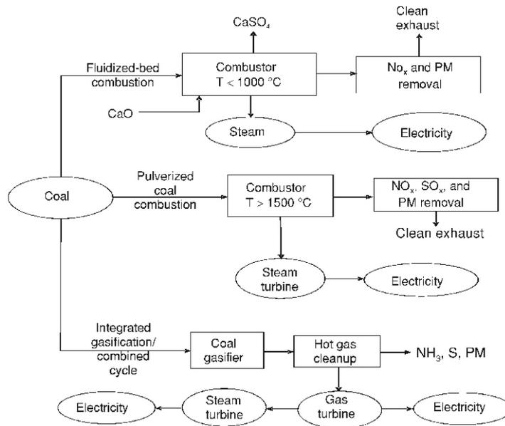
**Figure 2. Commercially available options for coal use in electricity production**
