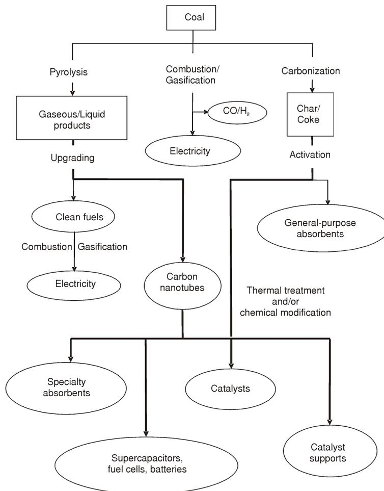
**Figure 3. Flow diagram of a vertically integrated coal complex**
